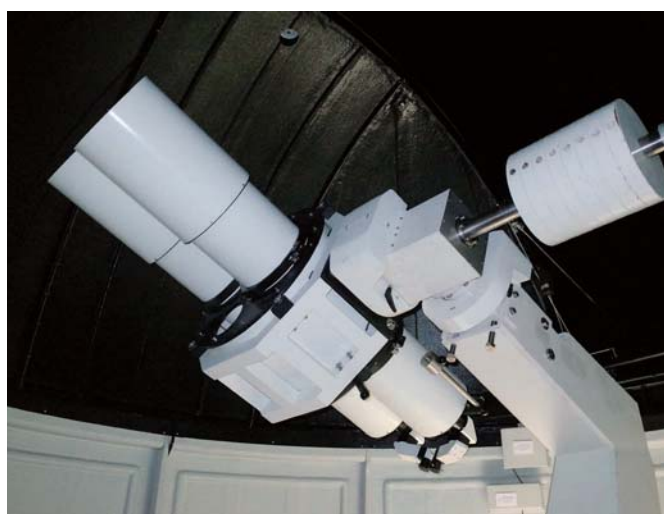
為兩位騰訊控股創辦人設計及建造，全球最大口徑 304 f7.5 APO 雙筒折射鏡 Designed and constructed for the two co-founders of Tencent Holdings, the world's largest 304mm f/7.5 APO binocular telescopes
