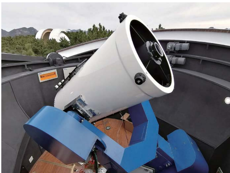
為中國科學院河北基地開發的 0.6 米口徑 f/2.15 大像場直焦望遠鏡 0.6m f/2.15 Prime focus reflector telescope designed and built for Hebei station, Chinese Academy of Sciences.
